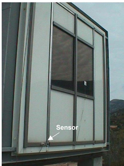
**Open loop control, the sensor is located outside of the controlled zone.**
