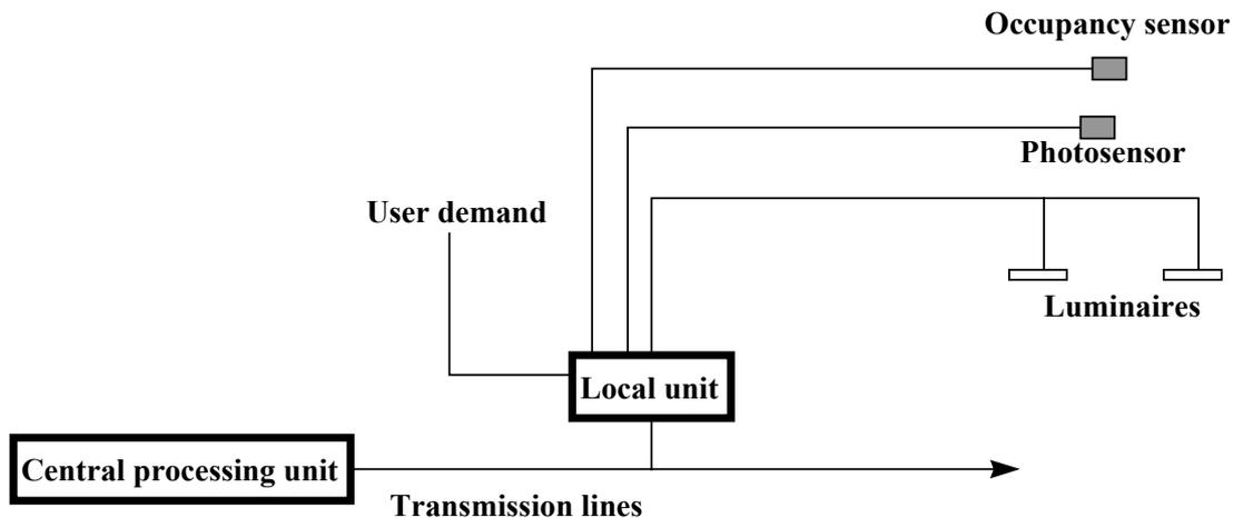
**Layout of control system for artificial lighting**
