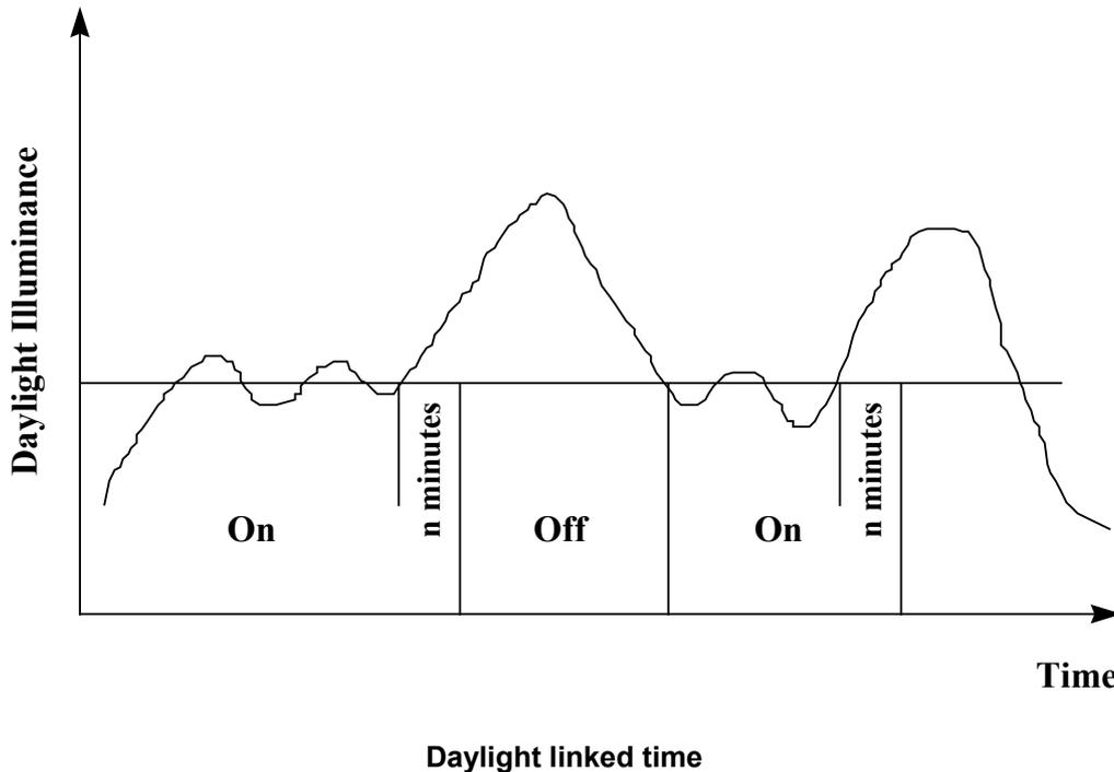
Of the two above mentioned time delay strategies, the second one gives significantly less switching. For the same time delay, the switching linked control will give lower energy use than the daylight linked version.
